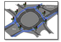
cyclists and pedestrians, connected to off-carriageway bike lanes for all directions. The pavement areas are enlarged and sharper turns are created for motor vehicles to reduce speeds.
